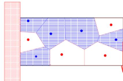
Fig. 2. Example of an indirect representation: Voronoi representation for the 2x1 cantilever test problem [15].
