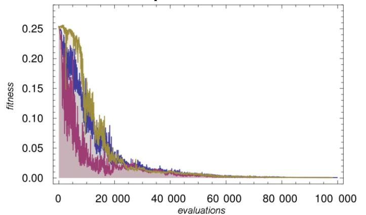
Fig. 8. Plot of three different evolutionary runs showing the fitness of both shapes (and their average) against the number of evaluations. The first case was unsuccessful, second case evolved only one fix-point, while the third case evolved both fix-points.
